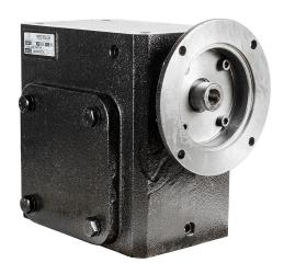
IronHorse heavy-duty worm gearbox, 40:1 ratio, 56C-Face input, right hand, 1.375in diameter output shaft, nominal 2hp at 1.0 SF, 3692 lb-in mechanical output torque, 3-1/4in center distance, cast iron housing, tapped-base mount.
