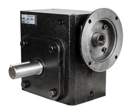
IronHorse heavy-duty worm gearbox, 40:1 ratio, 145TC-Face input, left hand, 1.375in diameter output shaft, nominal 2hp at 1.0 SF, 3692 lb-in mechanical output torque, 3-1/4in center distance, cast iron housing, tapped-base mount.
