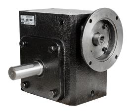
IronHorse heavy-duty worm gearbox, 40:1 ratio, 56C-Face input, left hand, 1.375in diameter output shaft, nominal 2hp at 1.0 SF, 3692 lb-in mechanical output torque, 3-1/4in center distance, cast iron housing, tapped-base mount.
