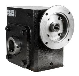
IronHorse heavy-duty worm gearbox, 40:1 ratio, 145TC-Face input, hollow, 1.937in diameter output shaft, nominal 2hp at 1.0 SF, 3692 lb-in mechanical output torque, 3-1/4in center distance, cast iron housing, tapped-base mount.
