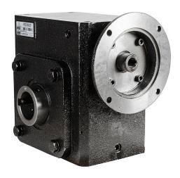
IronHorse heavy-duty worm gearbox, 40:1 ratio, 56C-Face input, hollow, 1.937in diameter output shaft, nominal 2hp at 1.0 SF, 3692 lb-in mechanical output torque, 3-1/4in center distance, cast iron housing, tapped-base mount.
