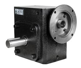
IronHorse heavy-duty worm gearbox, 40:1 ratio, 145TC-Face input, dual, 1.375in diameter output shaft, nominal 2hp at 1.0 SF, 3692 lb-in mechanical output torque, 3-1/4in center distance, cast iron housing, tapped-base mount.
