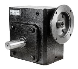
IronHorse heavy-duty worm gearbox, 40:1 ratio, 56C-Face input, dual, 1.375in diameter output shaft, nominal 2hp at 1.0 SF, 3692 lb-in mechanical output torque, 3-1/4in center distance, cast iron housing, tapped-base mount.
