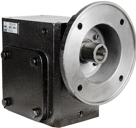
IronHorse heavy-duty worm gearbox, 30:1 ratio, 182TC-Face input, right hand, 1.375in diameter output shaft, nominal 3hp at 1.0 SF, 3045 lb-in mechanical output torque, 3-1/4in center distance, cast iron housing, tapped-base mount.
