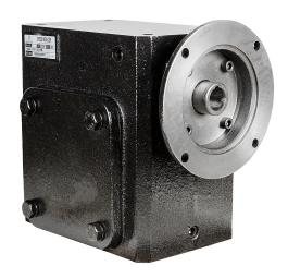
IronHorse heavy-duty worm gearbox, 30:1 ratio, 145TC-Face input, right hand, 1.375in diameter output shaft, nominal 2hp at 1.0 SF, 3045 lb-in mechanical output torque, 3-1/4in center distance, cast iron housing, tapped-base mount.
