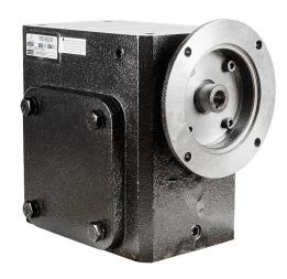
IronHorse heavy-duty worm gearbox, 30:1 ratio, 56C-Face input, right hand, 1.375in diameter output shaft, nominal 2hp at 1.0 SF, 3045 lb-in mechanical output torque, 3-1/4in center distance, cast iron housing, tapped-base mount.
