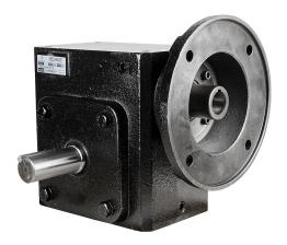
IronHorse heavy-duty worm gearbox, 30:1 ratio, 182TC-Face input, left hand, 1.375in diameter output shaft, nominal 3hp at 1.0 SF, 3045 lb-in mechanical output torque, 3-1/4in center distance, cast iron housing, tapped-base mount.
