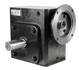
IronHorse heavy-duty worm gearbox, 30:1 ratio, 145TC-Face input, left hand, 1.375in diameter output shaft, nominal 2hp at 1.0 SF, 3045 lb-in mechanical output torque, 3-1/4in center distance, cast iron housing, tapped-base mount.
