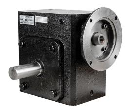
IronHorse heavy-duty worm gearbox, 30:1 ratio, 56C-Face input, left hand, 1.375in diameter output shaft, nominal 2hp at 1.0 SF, 3045 lb-in mechanical output torque, 3-1/4in center distance, cast iron housing, tapped-base mount.
