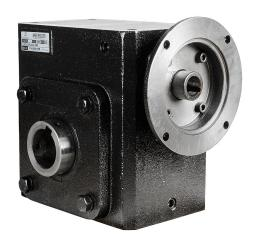
IronHorse heavy-duty worm gearbox, 30:1 ratio, 145TC-Face input, hollow, 1.937in diameter output shaft, nominal 2hp at 1.0 SF, 3045 lb-in mechanical output torque, 3-1/4in center distance, cast iron housing, tapped-base mount.
