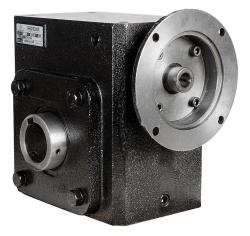
IronHorse heavy-duty worm gearbox, 30:1 ratio, 56C-Face input, hollow, 1.937in diameter output shaft, nominal 2hp at 1.0 SF, 3045 lb-in mechanical output torque, 3-1/4in center distance, cast iron housing, tapped-base mount.
