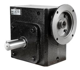
IronHorse heavy-duty worm gearbox, 30:1 ratio, 145TC-Face input, dual, 1.375in diameter output shaft, nominal 2hp at 1.0 SF, 3045 lb-in mechanical output torque, 3-1/4in center distance, cast iron housing, tapped-base mount.
