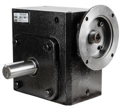
IronHorse heavy-duty worm gearbox, 30:1 ratio, 56C-Face input, dual, 1.375in diameter output shaft, nominal 2hp at 1.0 SF, 3045 lb-in mechanical output torque, 3-1/4in center distance, cast iron housing, tapped-base mount.
