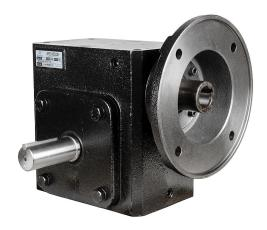
IronHorse heavy-duty worm gearbox, 20:1 ratio, 182TC-Face input, left hand, 1.375in diameter output shaft, nominal 3hp at 1.0 SF, 2875 lb-in mechanical output torque, 3-1/4in center distance, cast iron housing, tapped-base mount.
