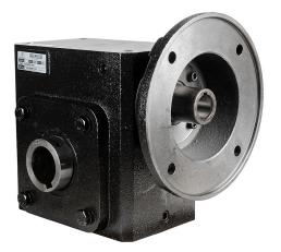
IronHorse heavy-duty worm gearbox, 20:1 ratio, 182TC-Face input, hollow, 1.937in diameter output shaft, nominal 3hp at 1.0 SF, 2875 lb-in mechanical output torque, 3-1/4in center distance, cast iron housing, tapped-base mount.
