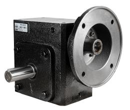
IronHorse heavy-duty worm gearbox, 20:1 ratio, 182TC-Face input, dual, 1.375in diameter output shaft, nominal 3hp at 1.0 SF, 2875 lb-in mechanical output torque, 3-1/4in center distance, cast iron housing, tapped-base mount.
