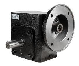
IronHorse heavy-duty worm gearbox, 20:1 ratio, 182TC-Face input, dual, 1.375in diameter output shaft, nominal 3hp at 1.0 SF, 2875 lb-in mechanical output torque, 3-1/4in center distance, cast iron housing, tapped-base mount.
