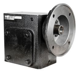
IronHorse heavy-duty worm gearbox, 15:1 ratio, 182/4TC-Face input, right hand, 1.375in diameter output shaft, nominal 5hp at 1.0 SF, 2611 lb-in mechanical output torque, 3-1/4in center distance, cast iron housing, tapped-base mount.
