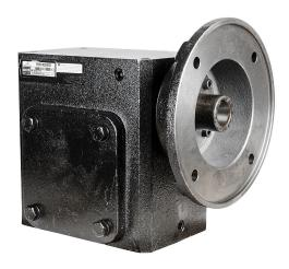
IronHorse heavy-duty worm gearbox, 15:1 ratio, 182/4TC-Face input, right hand, 1.375in diameter output shaft, nominal 5hp at 1.0 SF, 2611 lb-in mechanical output torque, 3-1/4in center distance, cast iron housing, tapped-base mount.
