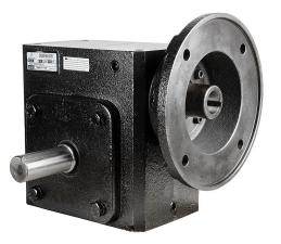
IronHorse heavy-duty worm gearbox, 15:1 ratio, 182/4TC-Face input, left hand, 1.375in diameter output shaft, nominal 5hp at 1.0 SF, 2611 lb-in mechanical output torque, 3-1/4in center distance, cast iron housing, tapped-base mount.
