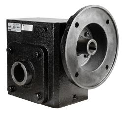
IronHorse heavy-duty worm gearbox, 15:1 ratio, 182/4TC-Face input, hollow, 1.937in diameter output shaft, nominal 5hp at 1.0 SF, 2611 lb-in mechanical output torque, 3-1/4in center distance, cast iron housing, tapped-base mount.
