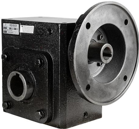
IronHorse heavy-duty worm gearbox, 15:1 ratio, 182/4TC-Face input, hollow, 1.937in diameter output shaft, nominal 5hp at 1.0 SF, 2611 lb-in mechanical output torque, 3-1/4in center distance, cast iron housing, tapped-base mount.
