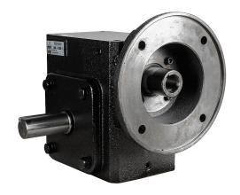
IronHorse heavy-duty worm gearbox, 15:1 ratio, 182/4TC-Face input, dual, 1.375in diameter output shaft, nominal 5hp at 1.0 SF, 2611 lb-in mechanical output torque, 3-1/4in center distance, cast iron housing, tapped-base mount.
