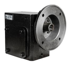
IronHorse heavy-duty worm gearbox, 10:1 ratio, 182/4TC-Face input, right hand, 1.375in diameter output shaft, nominal 5hp at 1.0 SF, 2419 lb-in mechanical output torque, 3-1/4in center distance, cast iron housing, tapped-base mount.
