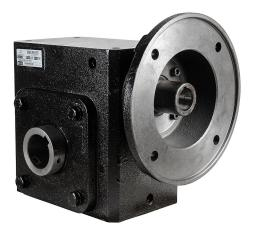
IronHorse heavy-duty worm gearbox, 10:1 ratio, 182/4TC-Face input, hollow, 1.937in diameter output shaft, nominal 5hp at 1.0 SF, 2419 lb-in mechanical output torque, 3-1/4in center distance, cast iron housing, tapped-base mount.
