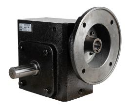
IronHorse heavy-duty worm gearbox, 10:1 ratio, 182/4TC-Face input, dual, 1.375in diameter output shaft, nominal 5hp at 1.0 SF, 2419 lb-in mechanical output torque, 3-1/4in center distance, cast iron housing, tapped-base mount.
