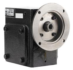
IronHorse heavy-duty worm gearbox, 60:1 ratio, 56C-Face input, right hand, 1.125in diameter output shaft, nominal 0.75hp at 1.0 SF, 1670 lb-in mechanical output torque, 2-5/8in center distance, cast iron housing, tapped-base mount.
