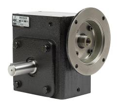
IronHorse heavy-duty worm gearbox, 60:1 ratio, 56C-Face input, left hand, 1.125in diameter output shaft, nominal 0.75hp at 1.0 SF, 1670 lb-in mechanical output torque, 2-5/8in center distance, cast iron housing, tapped-base mount.
