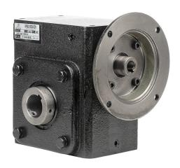
IronHorse heavy-duty worm gearbox, 60:1 ratio, 56C-Face input, hollow, 1.4375in diameter output shaft, nominal 0.75hp at 1.0 SF, 1670 lb-in mechanical output torque, 2-5/8in center distance, cast iron housing, tapped-base mount.
