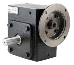
IronHorse heavy-duty worm gearbox, 60:1 ratio, 56C-Face input, dual, 1.125in diameter output shaft, nominal 0.75hp at 1.0 SF, 1670 lb-in mechanical output torque, 2-5/8in center distance, cast iron housing, tapped-base mount.
