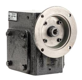
IronHorse heavy-duty worm gearbox, 40:1 ratio, 56C-Face input, right hand, 1.125in diameter output shaft, nominal 0.75hp at 1.0 SF, 1919 lb-in mechanical output torque, 2-5/8in center distance, cast iron housing, tapped-base mount.
