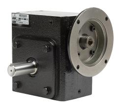
IronHorse heavy-duty worm gearbox, 40:1 ratio, 56C-Face input, left hand, 1.125in diameter output shaft, nominal 0.75hp at 1.0 SF, 1919 lb-in mechanical output torque, 2-5/8in center distance, cast iron housing, tapped-base mount.
