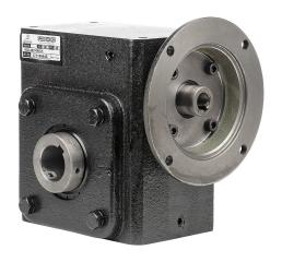
IronHorse heavy-duty worm gearbox, 40:1 ratio, 56C-Face input, hollow, 1.4375in diameter output shaft, nominal 0.75hp at 1.0 SF, 1919 lb-in mechanical output torque, 2-5/8in center distance, cast iron housing, tapped-base mount.
