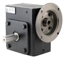
IronHorse heavy-duty worm gearbox, 40:1 ratio, 56C-Face input, dual, 1.125in diameter output shaft, nominal 0.75hp at 1.0 SF, 1919 lb-in mechanical output torque, 2-5/8in center distance, cast iron housing, tapped-base mount.
