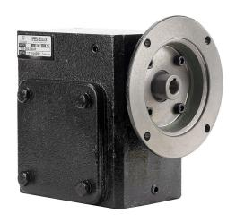
IronHorse heavy-duty worm gearbox, 20:1 ratio, 56C-Face input, right hand, 1.125in diameter output shaft, nominal 1.5hp at 1.0 SF, 1563 lb-in mechanical output torque, 2-5/8in center distance, cast iron housing, tapped-base mount.
