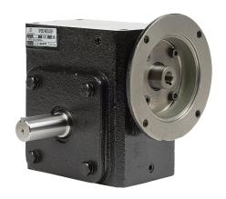
IronHorse heavy-duty worm gearbox, 20:1 ratio, 56C-Face input, left hand, 1.125in diameter output shaft, nominal 1.5hp at 1.0 SF, 1563 lb-in mechanical output torque, 2-5/8in center distance, cast iron housing, tapped-base mount.
