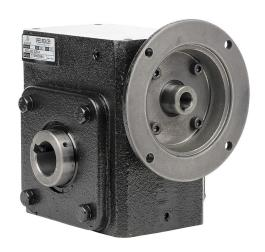
IronHorse heavy-duty worm gearbox, 20:1 ratio, 56C-Face input, hollow, 1.4375in diameter output shaft, nominal 1.5hp at 1.0 SF, 1563 lb-in mechanical output torque, 2-5/8in center distance, cast iron housing, tapped-base mount.
