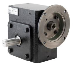
IronHorse heavy-duty worm gearbox, 20:1 ratio, 56C-Face input, dual, 1.125in diameter output shaft, nominal 1.5hp at 1.0 SF, 1563 lb-in mechanical output torque, 2-5/8in center distance, cast iron housing, tapped-base mount.
