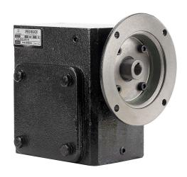
IronHorse heavy-duty worm gearbox, 15:1 ratio, 56C-Face input, right hand, 1.125in diameter output shaft, nominal 2hp at 1.0 SF, 1577 lb-in mechanical output torque, 2-5/8in center distance, cast iron housing, tapped-base mount.
