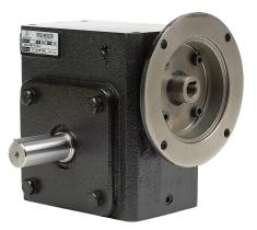
IronHorse heavy-duty worm gearbox, 15:1 ratio, 56C-Face input, left hand, 1.125in diameter output shaft, nominal 2hp at 1.0 SF, 1577 lb-in mechanical output torque, 2-5/8in center distance, cast iron housing, tapped-base mount.
