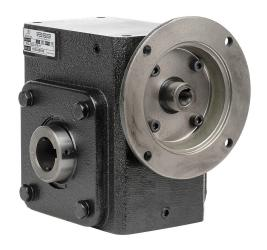
IronHorse heavy-duty worm gearbox, 15:1 ratio, 56C-Face input, hollow, 1.4375in diameter output shaft, nominal 2hp at 1.0 SF, 1577 lb-in mechanical output torque, 2-5/8in center distance, cast iron housing, tapped-base mount.
