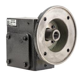
IronHorse heavy-duty worm gearbox, 10:1 ratio, 182TC-Face input, right hand, 1.125in diameter output shaft, nominal 2hp at 1.0 SF, 1445 lb-in mechanical output torque, 2-5/8in center distance, cast iron housing, tapped-base mount.
