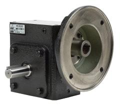
IronHorse heavy-duty worm gearbox, 10:1 ratio, 182TC-Face input, left hand, 1.125in diameter output shaft, nominal 2hp at 1.0 SF, 1445 lb-in mechanical output torque, 2-5/8in center distance, cast iron housing, tapped-base mount.
