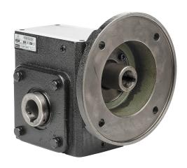
IronHorse heavy-duty worm gearbox, 10:1 ratio, 182TC-Face input, hollow, 1.4375in diameter output shaft, nominal 2hp at 1.0 SF, 1445 lb-in mechanical output torque, 2-5/8in center distance, cast iron housing, tapped-base mount.
