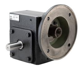
IronHorse heavy-duty worm gearbox, 10:1 ratio, 182TC-Face input, dual, 1.125in diameter output shaft, nominal 2hp at 1.0 SF, 1445 lb-in mechanical output torque, 2-5/8in center distance, cast iron housing, tapped-base mount.
