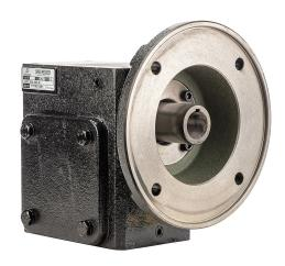
IronHorse heavy-duty worm gearbox, 5:1 ratio, 182TC-Face input, right hand, 1.125in diameter output shaft, nominal 3hp at 1.0 SF, 924 lb-in mechanical output torque, 2-5/8in center distance, cast iron housing, tapped-base mount.
