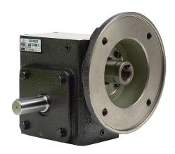
IronHorse heavy-duty worm gearbox, 5:1 ratio, 182TC-Face input, left hand, 1.125in diameter output shaft, nominal 3hp at 1.0 SF, 924 lb-in mechanical output torque, 2-5/8in center distance, cast iron housing, tapped-base mount.
