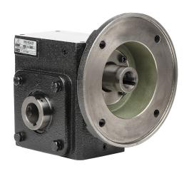
IronHorse heavy-duty worm gearbox, 5:1 ratio, 182TC-Face input, hollow, 1.4375in diameter output shaft, nominal 3hp at 1.0 SF, 924 lb-in mechanical output torque, 2-5/8in center distance, cast iron housing, tapped-base mount.
