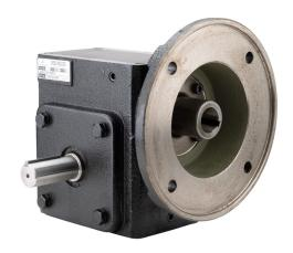
IronHorse heavy-duty worm gearbox, 5:1 ratio, 182TC-Face input, dual, 1.125in diameter output shaft, nominal 3hp at 1.0 SF, 924 lb-in mechanical output torque, 2-5/8in center distance, cast iron housing, tapped-base mount.
